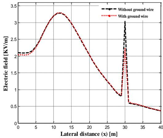
Figure 10. Electric field profile at 1 m above the ground with and without the ground wire
