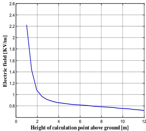
Figure 16. Variation of the perturbed electric field strength by varying the observation point above ground
