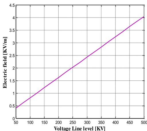
Figure 13. Variation of the perturbed electric field strength by varying the voltage level of transmission line
