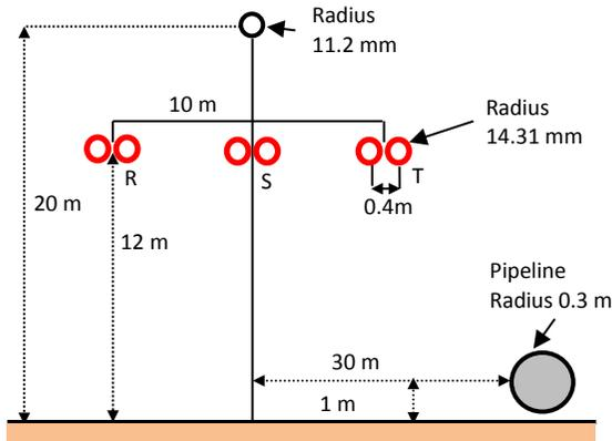
Figure 4. Single circuit horizontal configuration 275 kV with above pipeline
