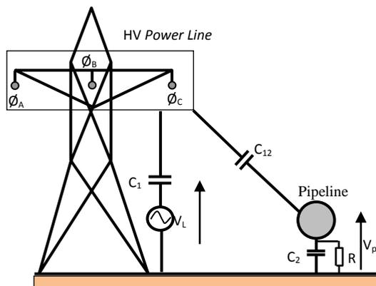
Figure 1. Capacitive coupling between pipeline and HV power line
