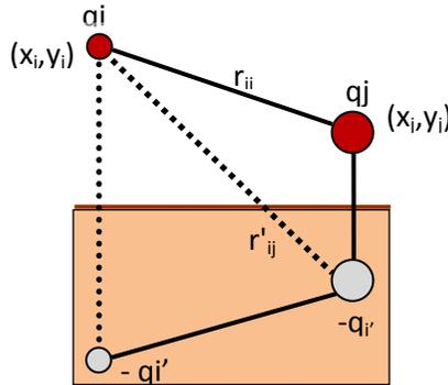
Figure 2. Determination of the potential coefficients for overhead lines
