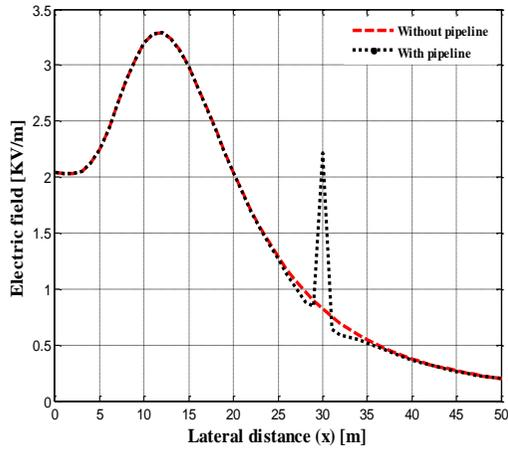
Figure 9. Electric field profile at 1 m above the ground with and without the pipeline
