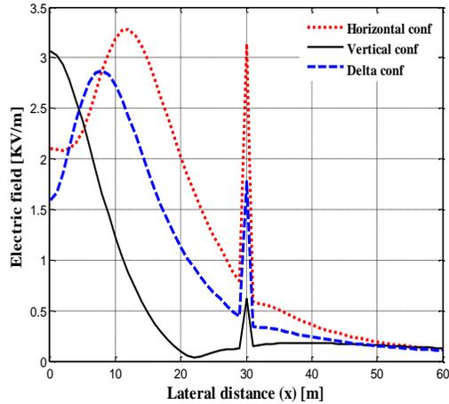
Figure 17. Lateral profiles of the perturbed electric field at 1m above the ground for various phase configurations
