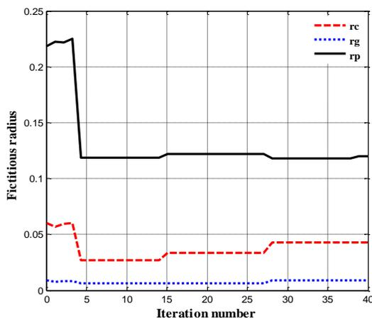
Figure 7. Convergence of the optimum values of fictitious charges radius ( $r_c$ ,  $r_g$ ,  $r_p$ )
