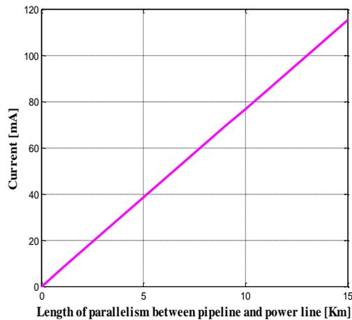
Figure 21. Relation between discharge current and the length of parallelism between HV line and pipeline
