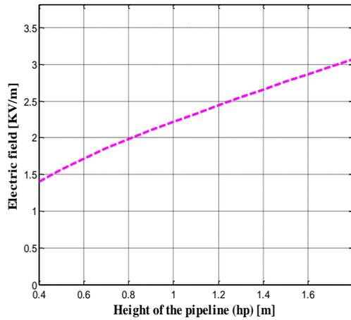
Figure 15. Variation of the perturbed electric field strength by varying the height of the pipeline above the ground
