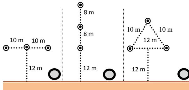
Figure 5. Different geometrical configurations for transmission overhead lines horizontal, (b) vertical, (c) delta
