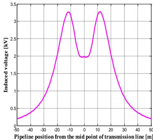
Figure 18. Induced voltage on the insulated pipeline due to 275 kV transmission line
