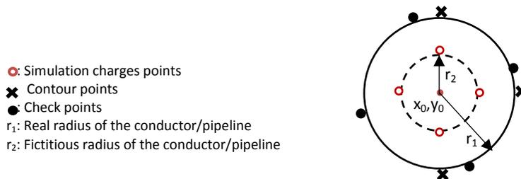
Figure 3. 2-D arrangement of simulation charges and contour points for the line (Conductor/ Pipeline)
