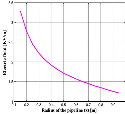
Figure 14. Variation of the electric field strength with pipeline radius
