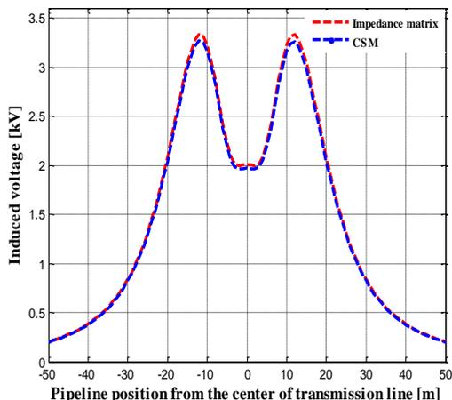
Figure 22. Comparison of induced voltage distribution between CSM+GA and the impedance matrix technique
