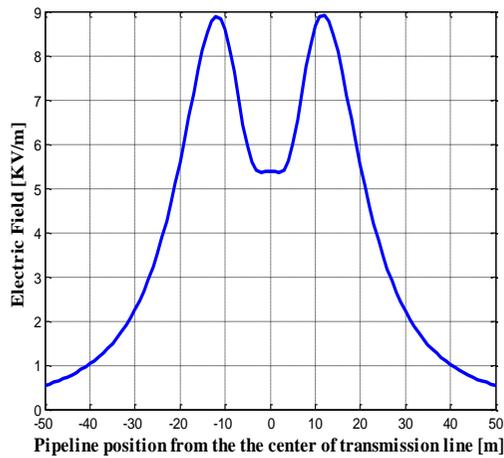
Figure 11. Perturbed electric field profile on the pipeline at 1 m above the the ground
