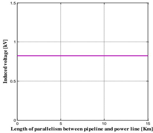
Figure 19. Relation between induced voltage and the length of parallelism between HV line and pipeline
