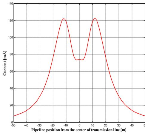
Figure 20. Discharge current profile passing through the human body
