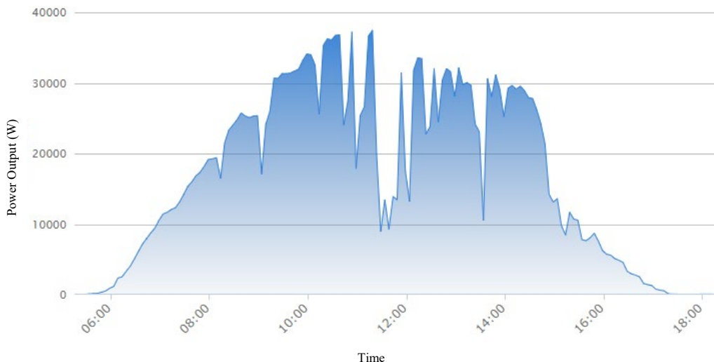
Figure 8. Actual power output from Duren Tiga grid-connected photovoltaic system.
