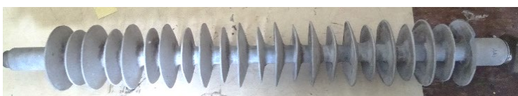
Figure 1. 30 Years-In-Service 70 kV Polymeric Insulator
