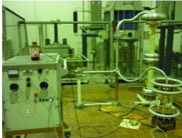
Figure 6. Arcing test circuit set-up
