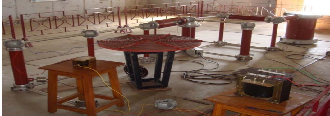
Figure 7. Snapshot of Test Setup of HFHV Layout Implemented for Composite Insulation Studies
