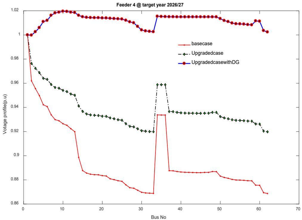
Figure 3. Voltage Profile of feeder F4 for different cases
