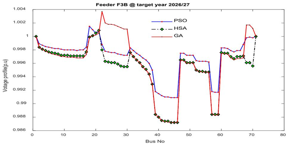
Figure 5. Voltage profile of separate upgraded feeder F3B for PSO, GA and HAS
