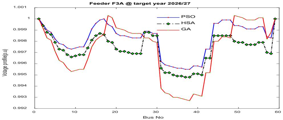
Figure 4. Voltage profile of separate upgraded feeder F3A for PSO, GA and HAS
