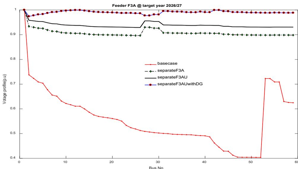
Figure 1. Voltage Profile of separated feeder F3A for different cases
