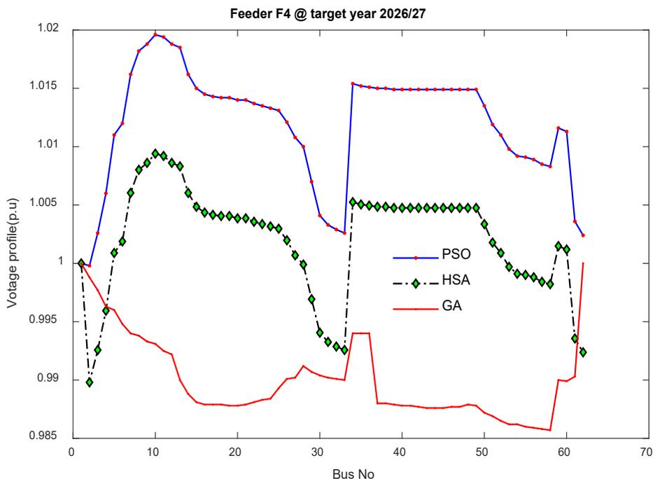
Figure 6. Voltage profile of separate upgraded feeder F4 for PSO, GA and HAS
