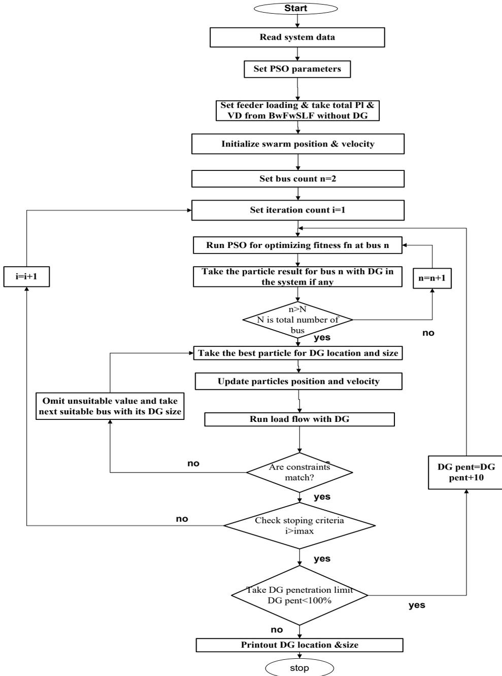
Figure 1. PSO algorithm for DG sizing and placement of DG penetration determination
