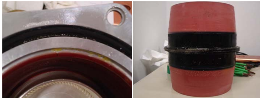
Figure 13 busbar socket with pollutants
