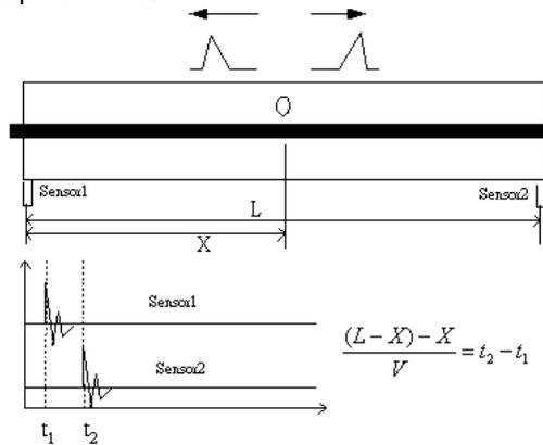
Figure 5. Diagram of time flying method
