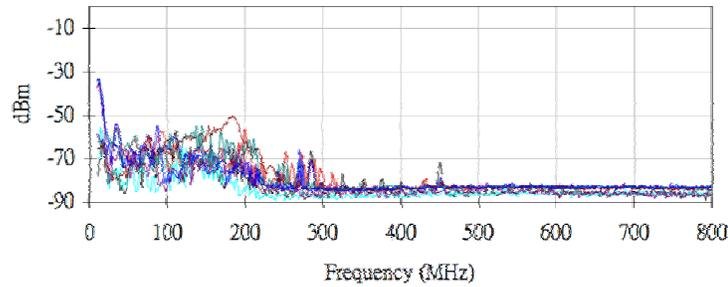
Figure 3. Background noises measured at MV substations in semiconductor manufactories
