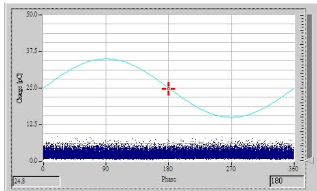
Figure 14. Phase-resolved pattern of on-line PDM on CGIS
