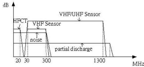
Figure 4. Spectrums of signals and PD sensors
