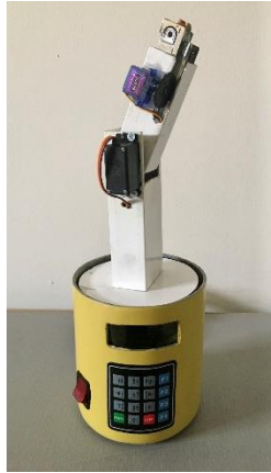
Figure 6. Experimental two-DOF gimbal system
