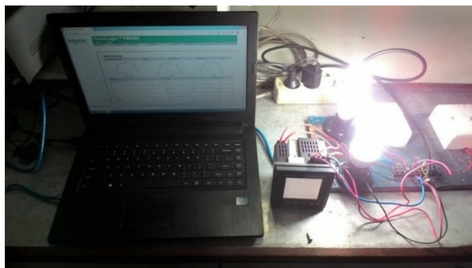
Figure 10. Configuration and Measurement of Non-Linear Load (Energy-Saving Lamps).
