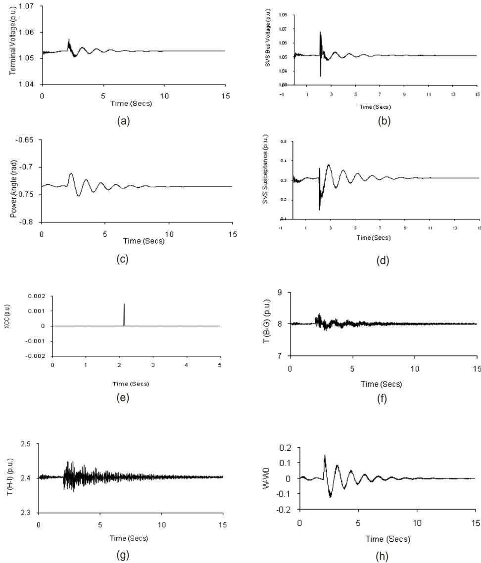
Figure 10(a-h). Response curves with CDRPDCIV auxiliary controller and controlled series compensation at  $P_g = 800$  MW due to 20% increase in  $T_{mech}$  for 0.1 secs (T-circuit Model)
