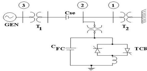
Figure 1. Electrical Network with SVS
