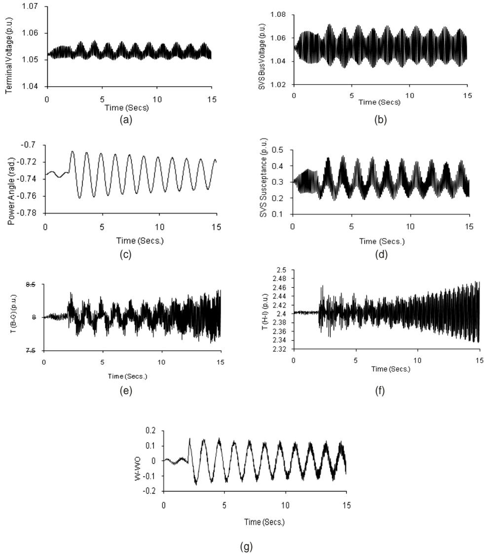
Figure 8(a-g). Response curves without CDRPDCIV auxiliary controller at  $P_g = 800$  MW due to 20% increase in  $T_{mech}$  for 0.1 secs (T-circuit Model)
