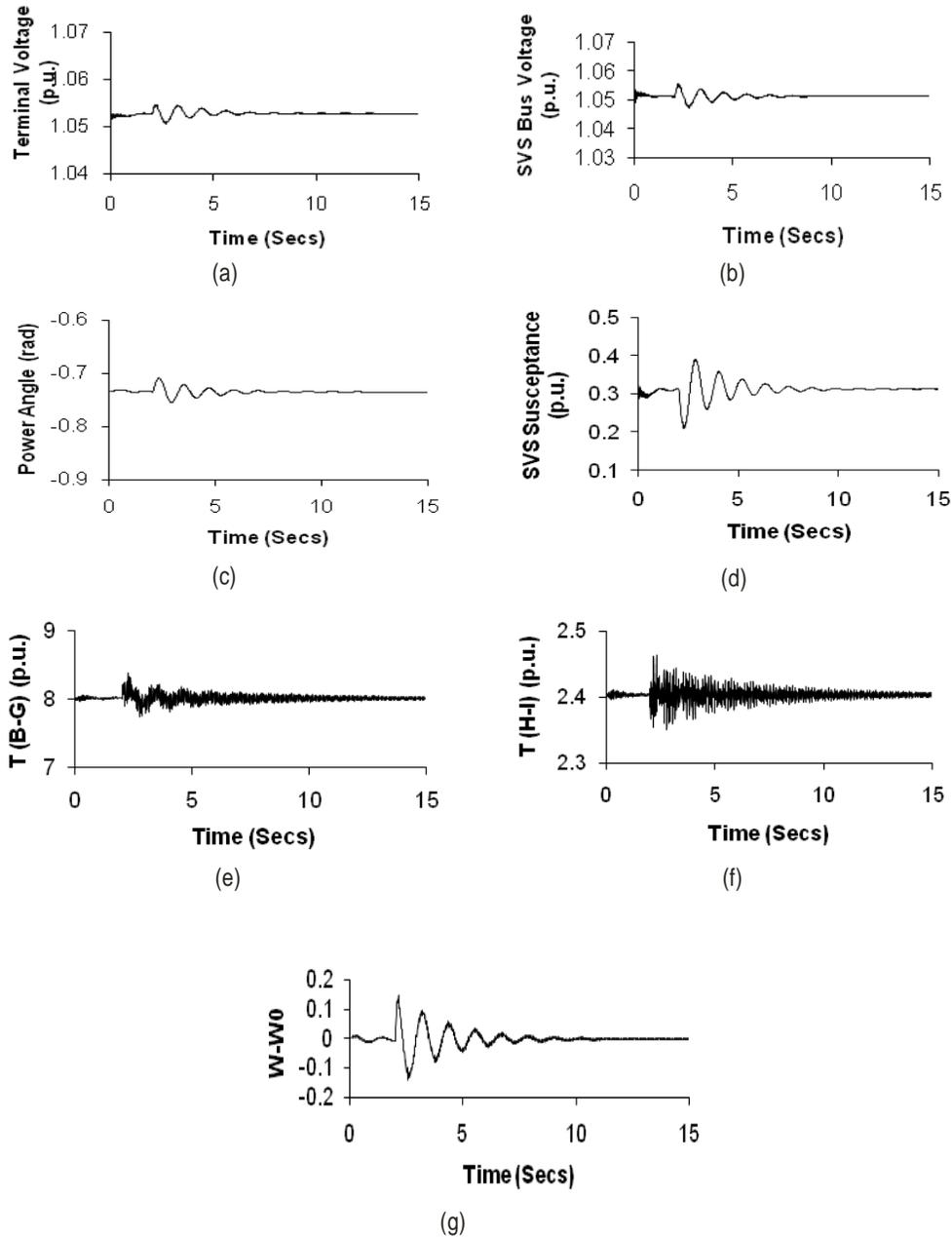
Figure 9(a-g). Response curves with CDRPDCIV auxiliary controller at  $P_g = 800$  MW due to 20% increase in  $T_{mech}$  for 0.1 secs (T-circuit Model)
