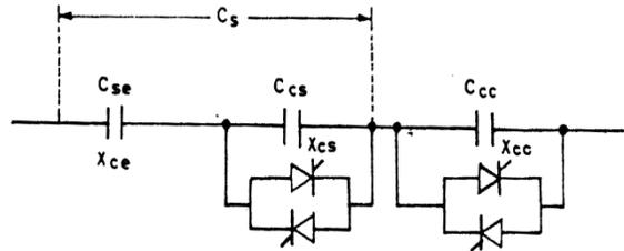
Figure 7. Controlled series compensation scheme
