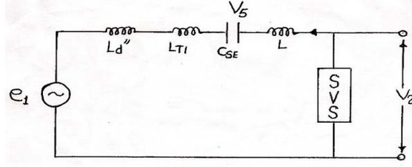
Figure 6.  $\alpha$ -axis representation of simplified system for DCIV signal
