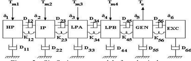
Figure 2. Six-Spring mass model of mechanical system
