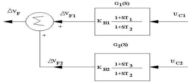
Figure 5. Control scheme for (CDR.PDCIV) auxiliary controller
