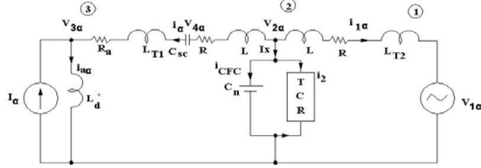
Figure 3.  $\alpha$ - axis representation of the network
