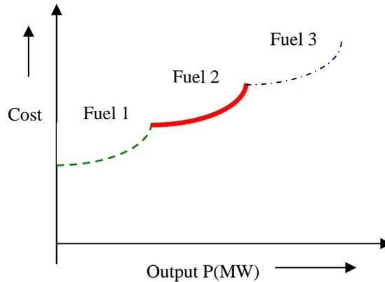
Figure 2.2. Fuel Cost Function Supplied with Multiple Fuel Types
