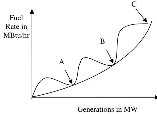
Figure 2.1. Valve point curve
