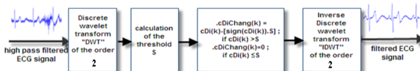
Figure 5. The high frequencies filter block diagram, cD_i is the detail coefficients of DWT.
