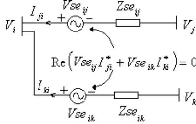
Figure 2. Equivalent circuit of two converter IPFC
