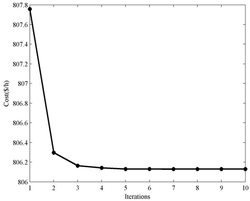
Figure 6. Convergence characteristics of IEEE 30 bus system using ISEA with IPFC.
