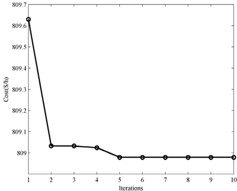
Figure 5. Convergence characteristics of IEEE 30 bus system using ISEA without IPFC.
