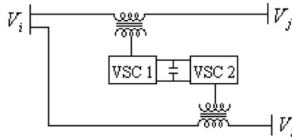
Figure 1. Schematic diagram of two converter IPFC
