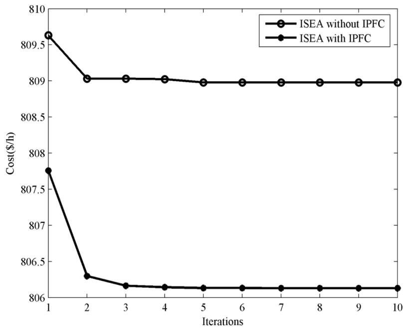
Figure 7. Convergence characteristics of IEEE 30 bus system using ISEA without & with IPFC
