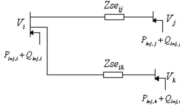
Figure 3. Power injection model of two converter IPFC
