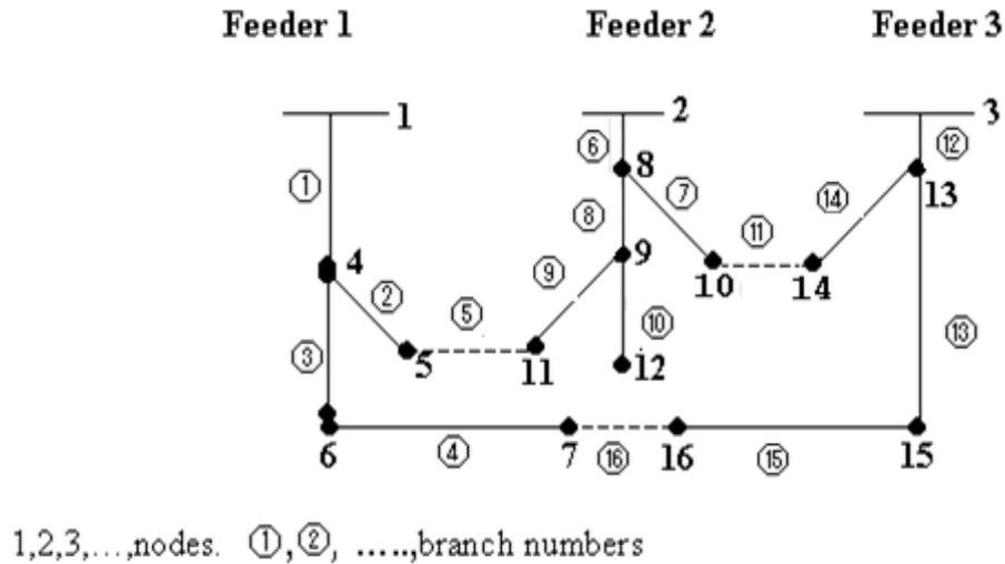
Figure 2. Single line diagram of IEEE 16-node system
