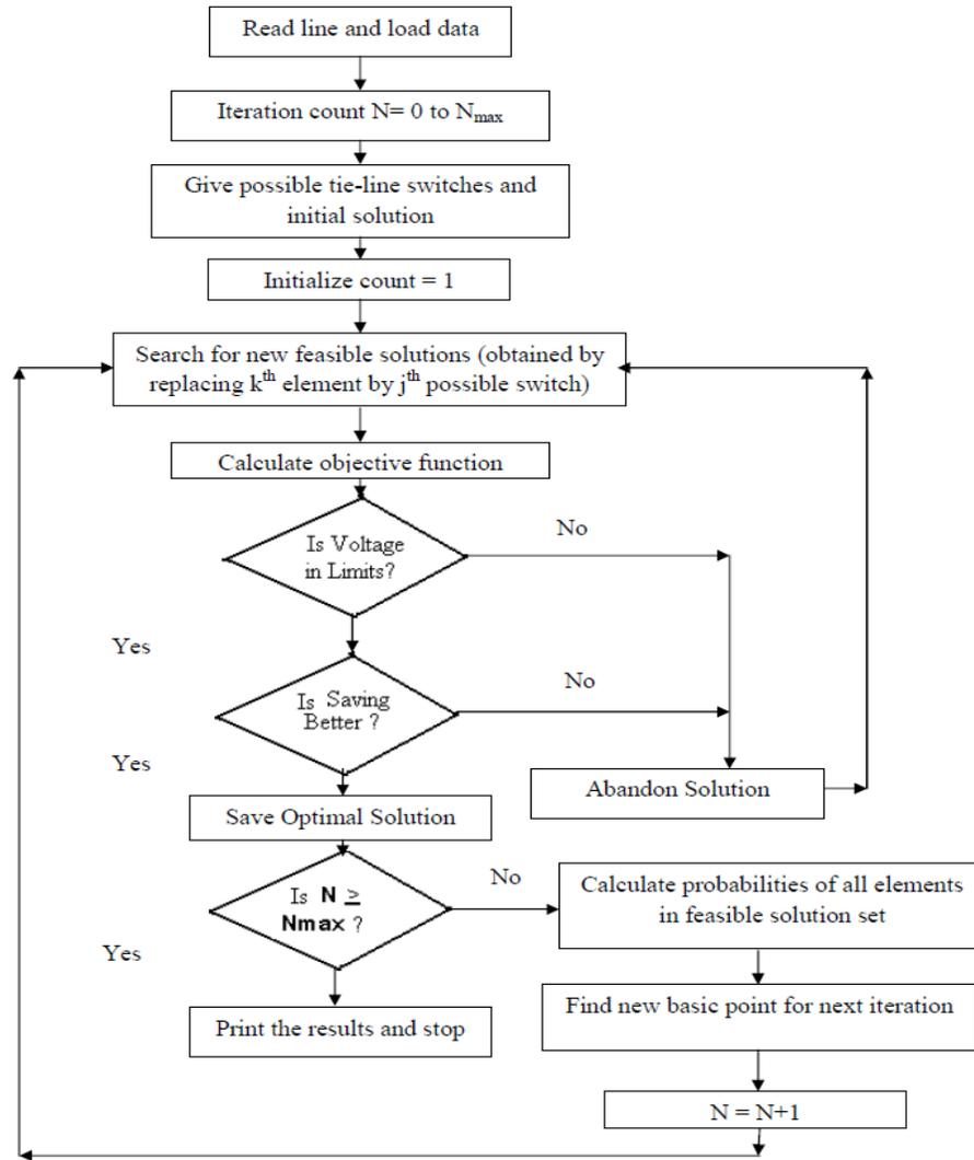
Figure 3. Flow Chart for network reconfiguration using PGSA
