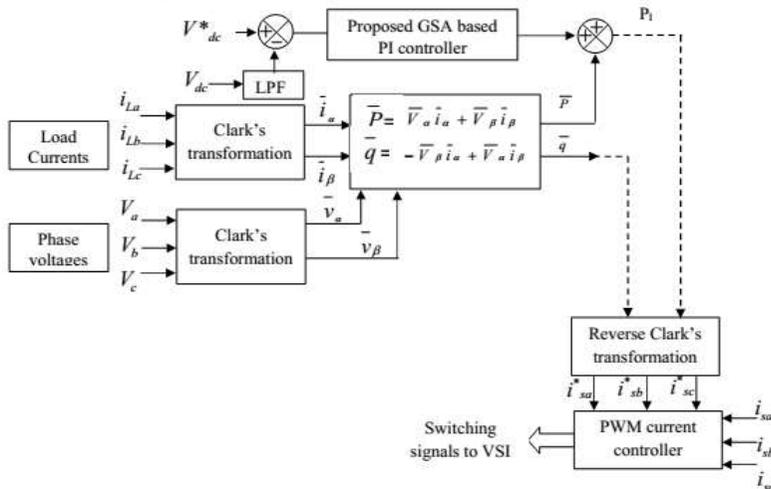
Figure 2. Proposed method based instantaneous reactive power theory
