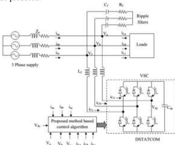
Figure 1. Block diagram of proposed method based D-STATCOM
