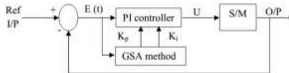
Figure 3. Gain tuning of PI controller using proposed method
