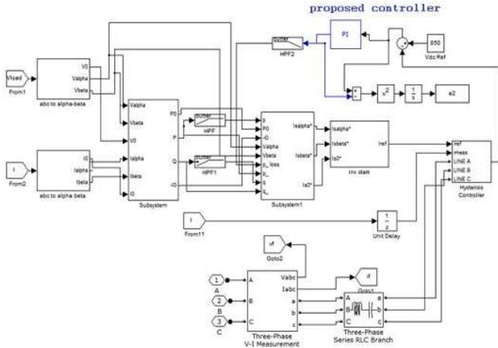
Figure 5. Simulink model of the proposed method based D-STATCOM
