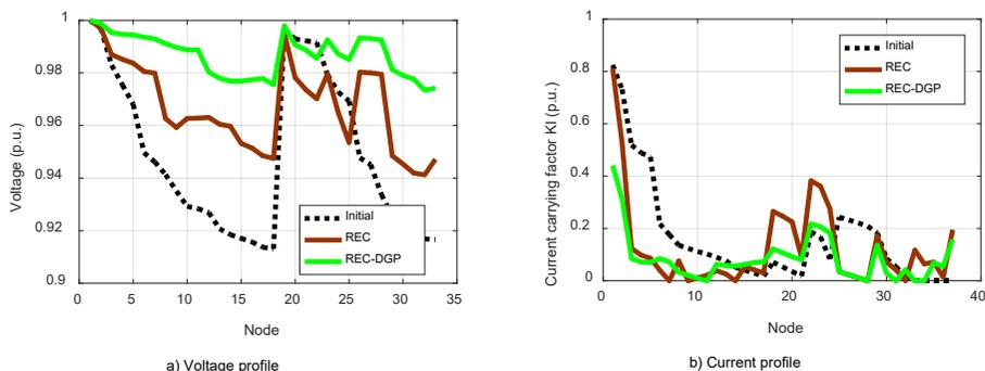
Figure 4. Voltage amplitude profile for the 33-node system by REC and REC-DGP
