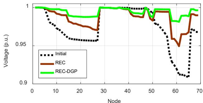
Figure 7. Voltage amplitude profile for the 69-node system by REC and REC-DGP
