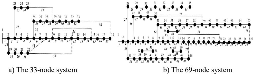
Figure 3. The 33-node and 69-node systems
