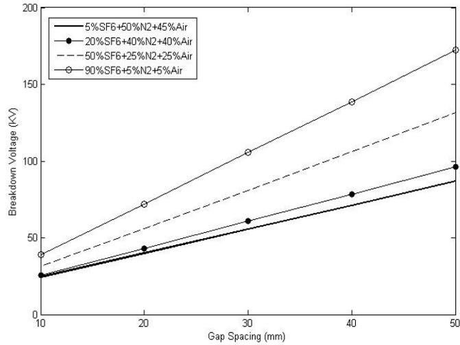
Figure 18. Effect of gap spacing on Breakdown Voltage for SF<sub>6</sub>:N<sub>2</sub>:Air gas mixture at P=300KPa
