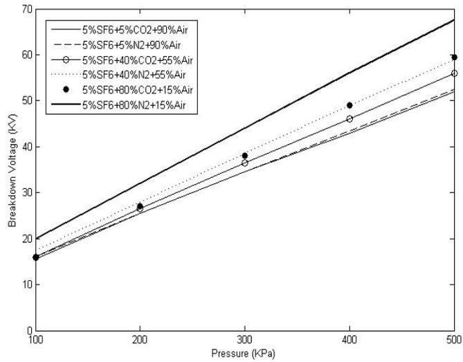
Figure 17. Effect of gas pressure for 5%SF<sub>6</sub>-gas mixture on Breakdown Voltage for a gap with particle contamination
