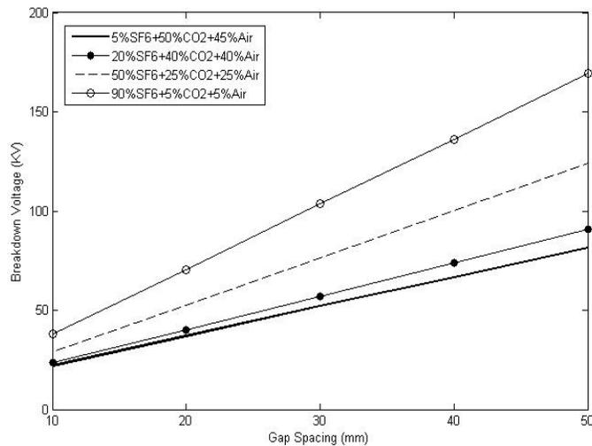
Figure 19. Effect of gap spacing on Breakdown Voltage for SF<sub>6</sub>:CO<sub>2</sub>:Air gas mixture at P=300KPa
