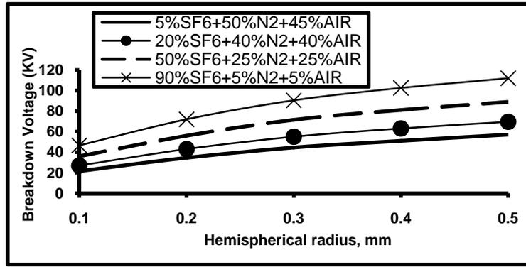
Figure 20. Effect of hemispherical radius of particle on Breakdown Voltage for SF<sub>6</sub>:N<sub>2</sub>:Air gas mixture at P=300KPa
