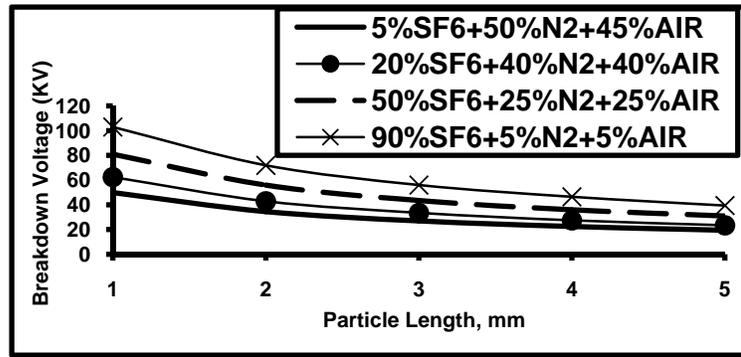
Figure 21. Effect of particle length on Breakdown Voltage for SF<sub>6</sub>:N<sub>2</sub>:Air gas mixture at P=300KPa
