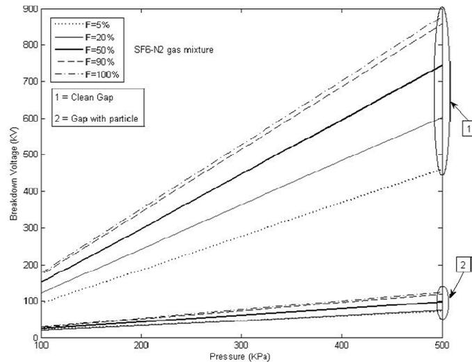
Figure 22. Effect of gas pressure on breakdown voltage for clean gap and gap with particle contamination for a various fractional concentrations of SF<sub>6</sub>-N<sub>2</sub> gas mixture
