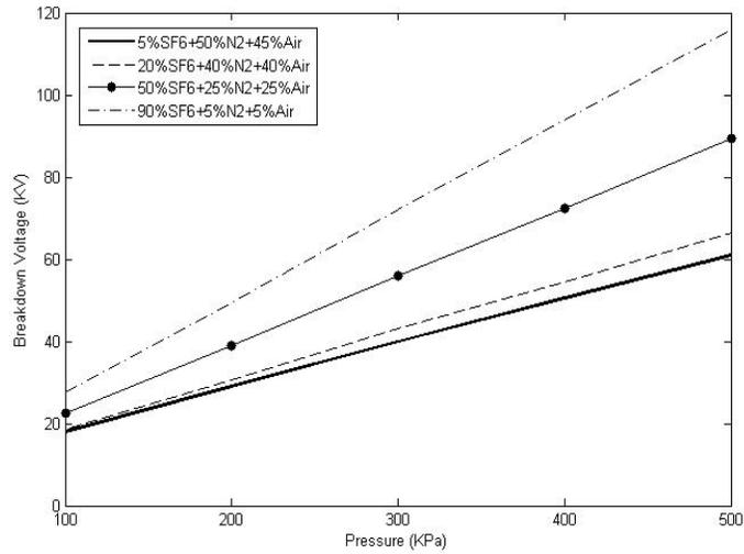
Figure 16. Effect of gas pressure for SF<sub>6</sub>:N<sub>2</sub>:Air mixture on Breakdown Voltage for a gap with particle contamination
